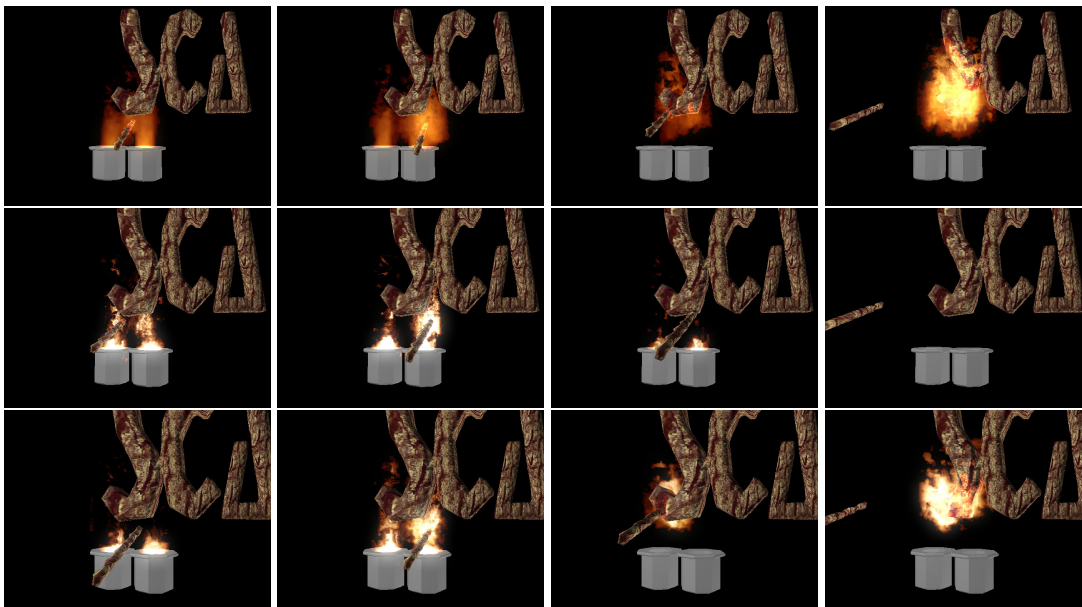
Figure 7. During the coarse resolution interactive simulation (top row), the user ignited a match and burned the conference logo. During higher resolution simulation (second row), the match barely lit, hence the logo did not burn at all. The controlled simulation (last row) injected additional combustible gas and heat into the system, and thus burned in a manner similar to that in the preview simulation. Note that the simulation control matches the fluid domain only, and hence does not have direct control on how the logo burns and decomposes.
