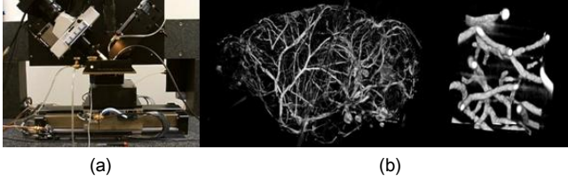
Fig. 2. (a) A full view of the Knife-Edge Scanning Microscope. (b) Sagittal section of whole mouse brain vasculature (left) and a close-up of a small part of it (right).
