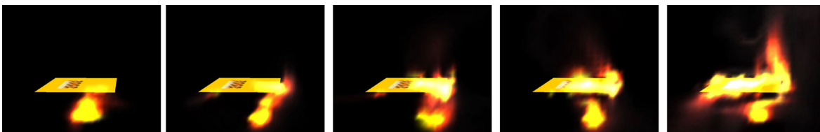
Figure 11. Self ignition of materials near a flame. As heat produced by the combustion rises, the paper begins pyrolysis, releasing fuel. This fuel also combusts, raising the temperature further and causing the flame to spread.
