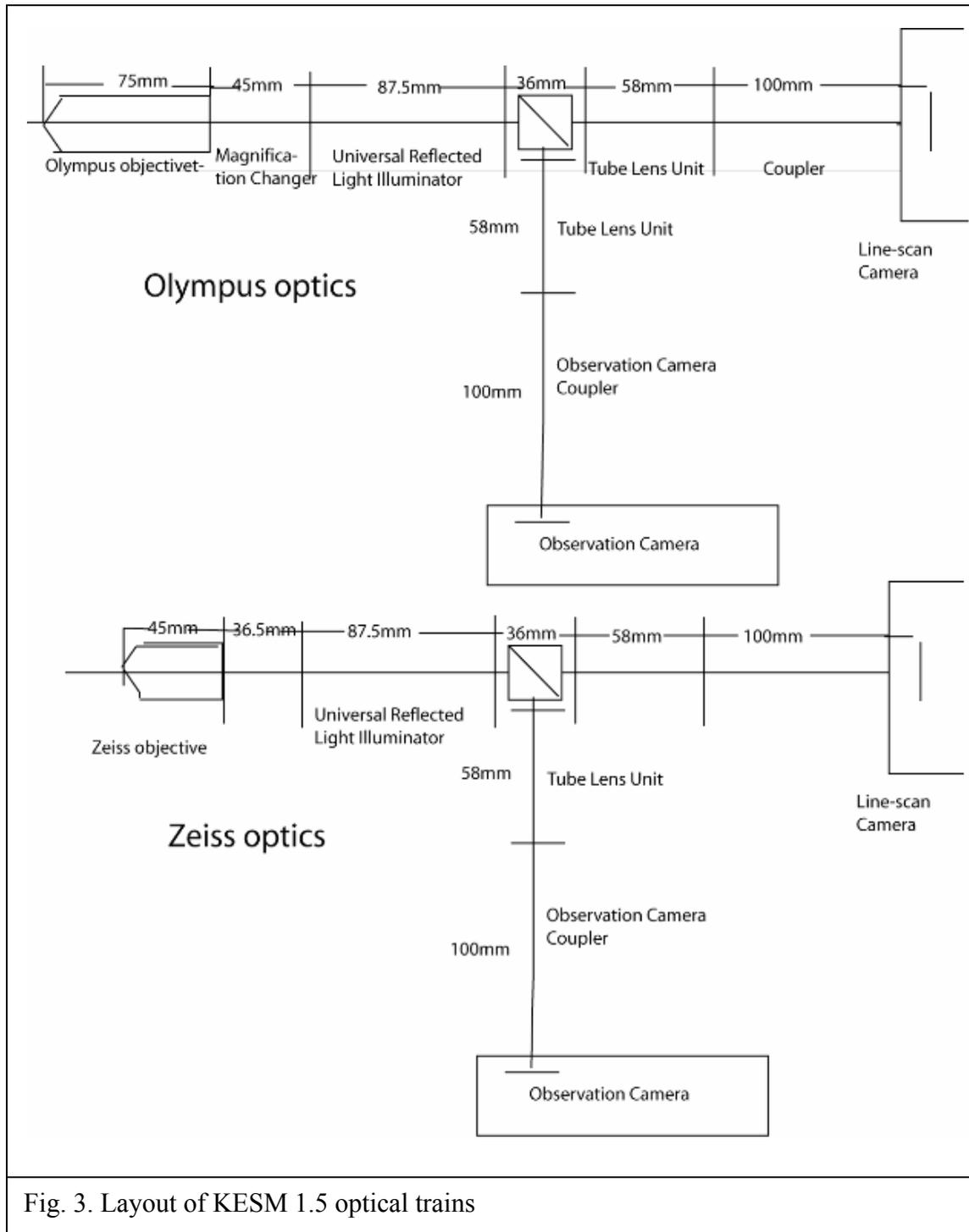
Fig. 3. Layout of KESM 1.5 optical trains
