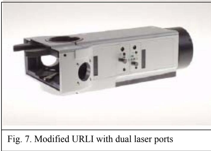
Fig. 7. Modified URLI with dual laser ports
